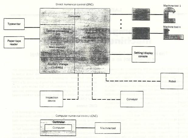
In its basic configuration, Fujitsu Fanuc's direct numerical control system K includes several numerically controlled machine tools connected to a central computer. With the connection of additional components such as robots, conveyors, and inspection
