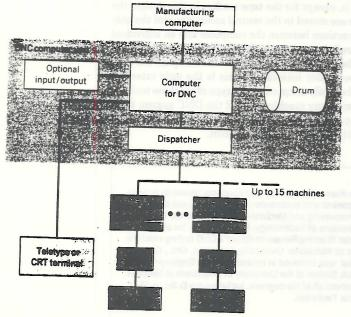
stored in the computer memory. When machining a part, the computer presents data in a format similar to that from the tape reader (but without pauses between blocks of information). This means that the part-data tape in such systems is used only once per manufaturing series, thus avoiding one of the biggest sources of error in NC systems.
