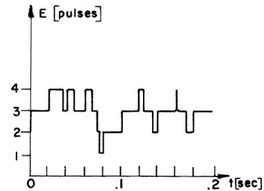
Fig. 7. Typical error at low velocity ( $K = 21$  s<sup>-1</sup>).
