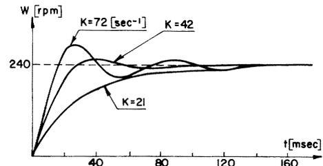
Fig. 6. Closed-loop response with the open-loop gain as parameter.
