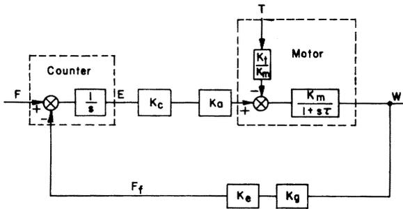
Fig. 3. Block diagram of the digital control loop.
