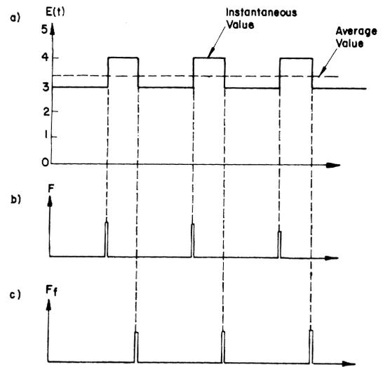
Fig. 2. The counter output for constant speed rotation.
