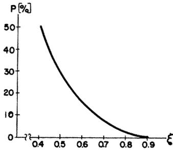
Fig. 4. The overshoot percentage of the counter versus damping factor.
