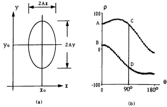
Fig. 4 Extraction of the parameters of an ellipse using Hough transform: (a) input ellipse image; (b) output image resulting from computing the Hough transform envelope, using a HT filter with impulse response for detection of a straight line in normal parameterization.
