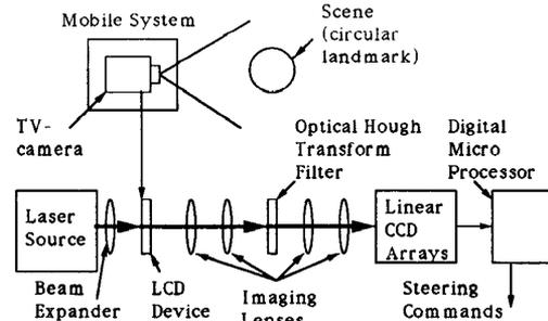
Fig. 3 Block diagram of the hybrid opto-electronic processor.
