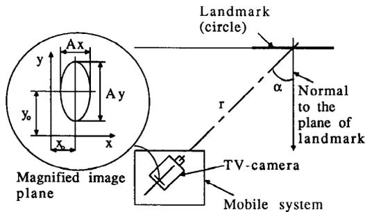
Fig. 1 Description of the relative spatial position of the mobile system and the landmark.
