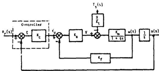
Fig. 6: Control loop using voltage amplifier
