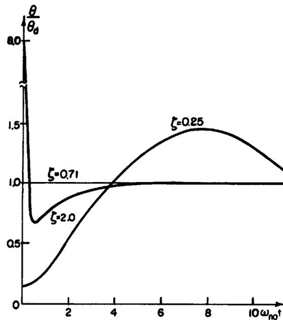
Fig 4: Position response of a misadjusted compensated torque loop to a step of  $\theta_d$
