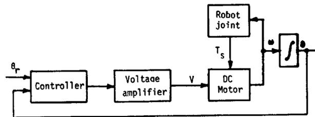
Fig. 2: Speed control of robot arm
