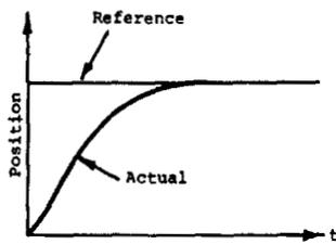
Fig. 7: Required and actual position response in a speed control loop
