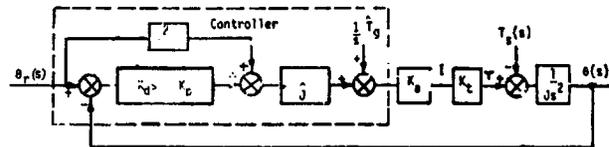
Fig. 3: Compensated torque control loop
