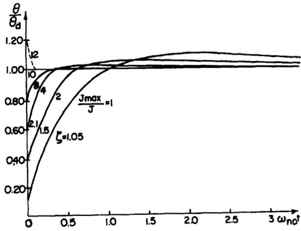
Fig. 5: Position response in a compensated loop adjusted according to the Min-Max method
